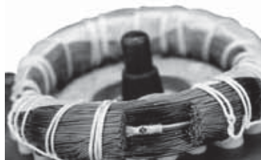
Fig. 28 PTC sensor incorporated in windings
