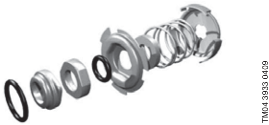
Fig. 10 Exploded view of shaft seal
