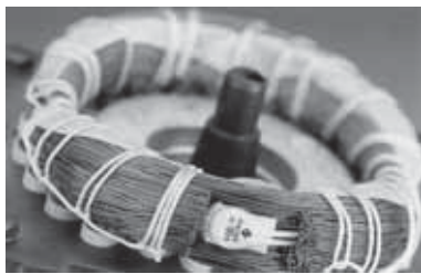
Fig. 30 Thermal switch incorporated in windings
